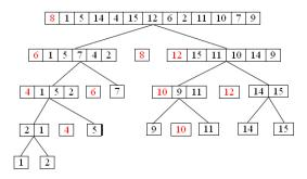
Solution: pick a pivot p uniformly at random (Las Vegas algorithm) Run time  $O(2n \log n)$
